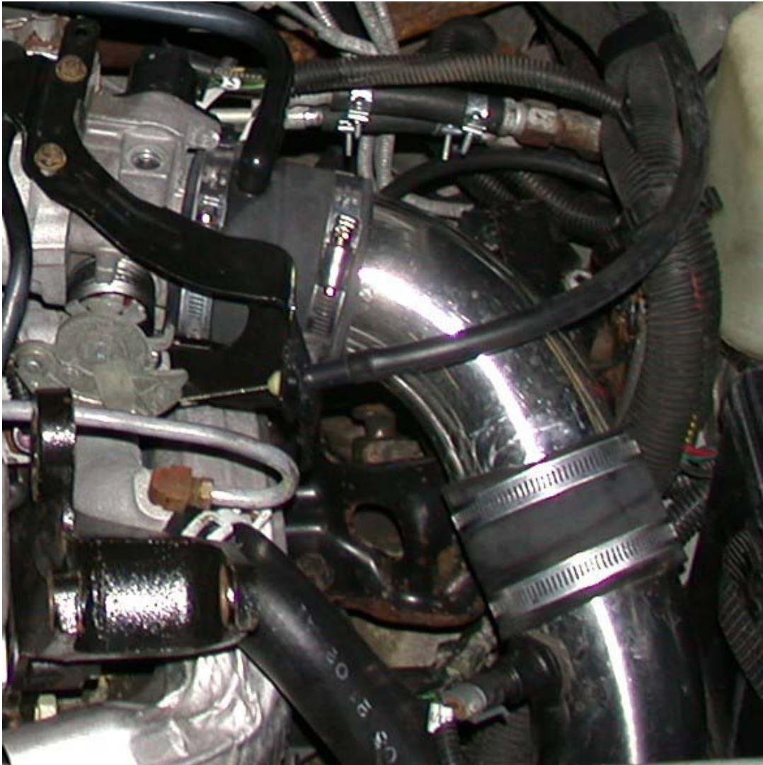
Custom cold air intake, please note the Intake air temperature sensor
