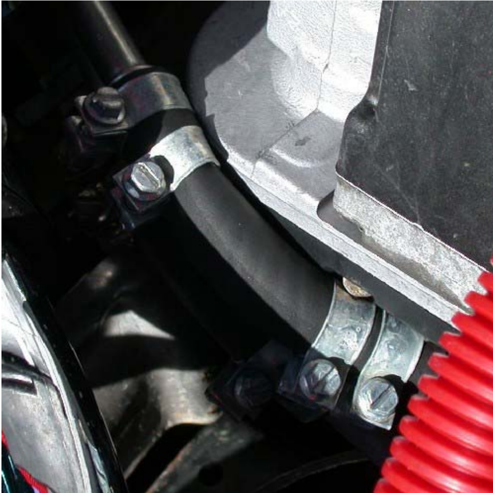
Double clamped fuel lines near Antilock Brake Master Cylinder
